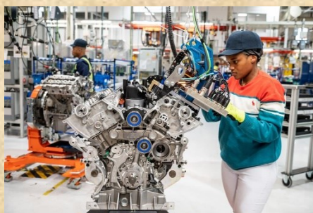
Ford Struandale Engine Plant – 3.0L V6 Diesel engine assembly in 2023.
